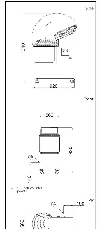
Electric Supply voltage: 380-415V/3 ph/50 Hz **Total Watts:** 2.2 kW Capacity: Maximum kneading (60% 50 kg/Cycle hydratation): Key Information: External dimensions, Width: 560 mm External dimensions, Depth: 880 mm External dimensions, Height: 830 mm 118 kg **Shipping weight: Bowl capacity:** 62 lt
